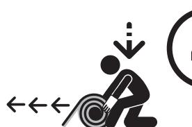
With the band(s) cut, maintain firm downward pressure on the mat. Start to gently release this pressure. Do this very slowly in small steps, allowing the mat to gradually expand and unroll.
