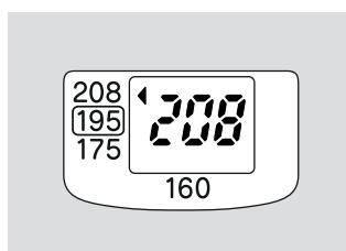
When the water temperature reaches 208°F, "208" appears on the Display.
