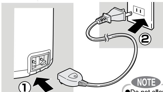
Be sure to insert the Power Cord securely. (Otherwise, may cause electric shock, short circuit, smoke or fire.)
