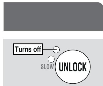
10 seconds after dispensing, the UNLOCK light turns off and the Automatic Dispense Lock is activated.
