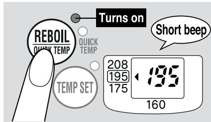
When the Reboil process is completed, the product switches to Keep Warm mode.
