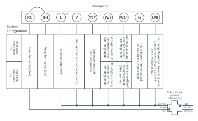
†Internal jumper between RC and RH, located on back of thermostat.
