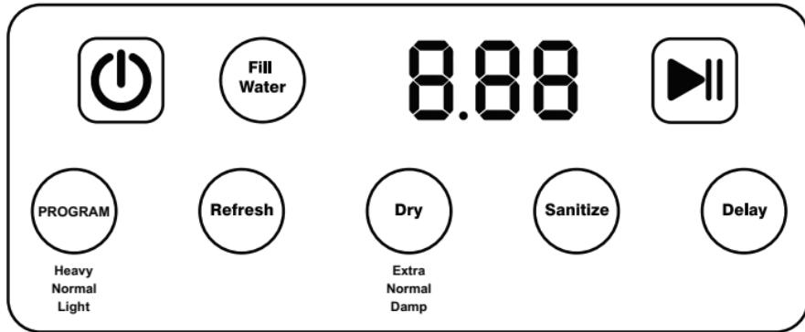
**On/O ffPower icon** - Powers on the Steam Dryer Closet. All the selections on the Control Panel illuminate.
