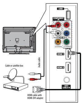
5 Connect an audio cable (not included) to the L/R AUDIO jacks on the side of your TV and to the AUDIO OUT jacks on the cable or satellite box.
