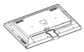
2 Make sure that the wide portion of the stand base faces the front of your TV, align the locators on the stand column with the locating grooves on the stand base, then secure the base to your TV with the base provided screws.
