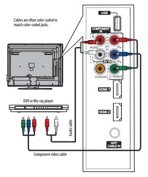
3 Connect an audio cable to the L/R AUDIO jacks on the side of your TV and to the L/R AUDIO OUT jacks on the component video device.
