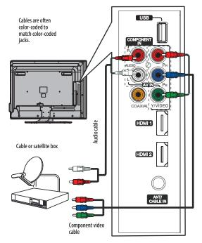
4 Connect an audio cable (not included) to the L/R AUDIO jacks on the side of your TV and to the audio out jacks on the cable or satellite TV box.
