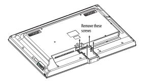
**3** Attach the wall-mount bracket to your TV using the mounting holes on the back of your TV. See the instructions that came with the wall-mount bracket for information about how to correctly hang your TV.
