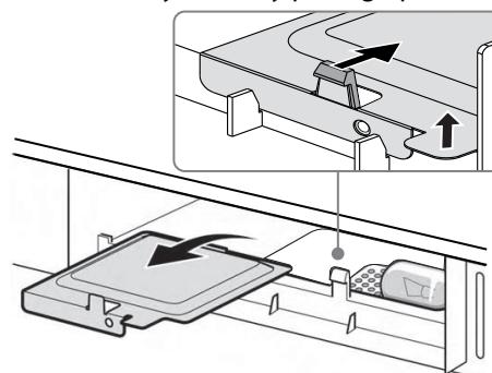
5 Remove the old light bulb and replace with a new, equivalent bulb. Do not use a bulb larger than 30W.
