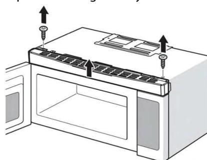
3 To remove the charcoal filter, push it inward, then lift it up and pull it away from the microwave.
