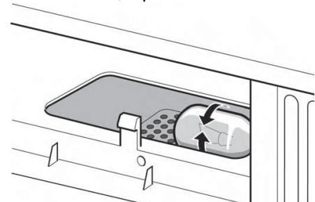
6 Push the light cover back into place and replace the charcoal filter.
