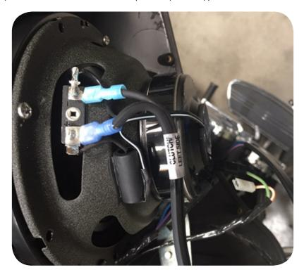
**STEP 8 -** Re-connect the positive (+) side of the battery, followed by the negative (-) side. **Warning:** Do not install the in-line fuse until after this step.
