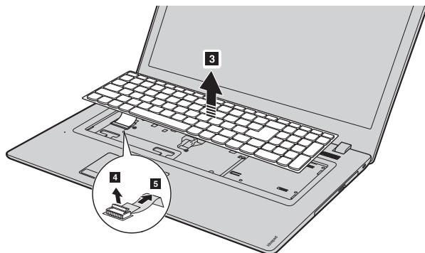
⑥ Reconnect the keyboard connector and install the new keyboard. Push the keyboard in gently until it clicks into place.
