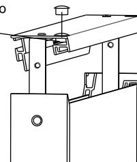
12. Remove all three screws on the opposite side of the hinge and carefully lift off the door latch assembly.
