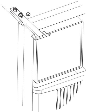
13. Place the door latch assembly on opposite side of unit.
