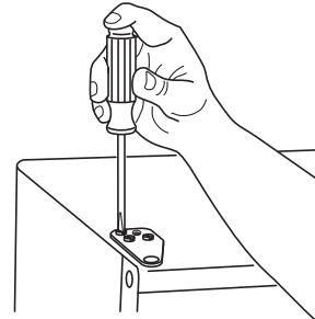
15. Adjust door to ensure proper seal. Tighten upper and lower hinge screws securely.
