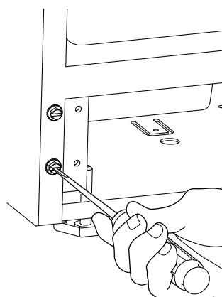
6. Install hinge on opposite side at bottom of cabinet. Align hinge outer edge with cabinet before tightening screws.
