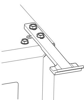
14. Place door on lower hinge pin. Invert and install upper hinge on door. Fasten upper hinge to unit (three screws). Partially tighten screws.
