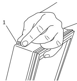
8. Using a Phillips screwdriver, remove the two screws holding the custom stainless handle from the original location and remove the handle. Remove the two screws on the opposite side of the door. Do not place handle on door until you have completed step 9.
