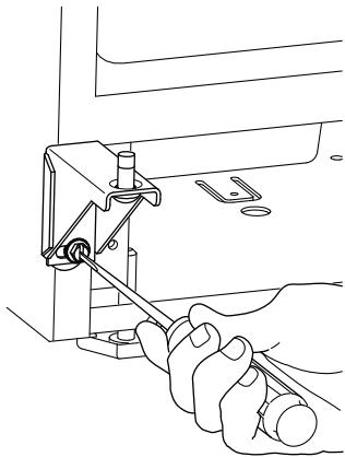
7. Relocate plastic spacer/bushing on top and bottom of door to opposite side. Clean out bushing hole in door bottom with a screwdriver if necessary.
