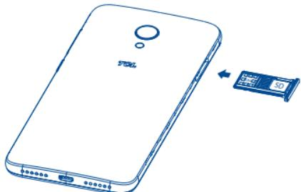
To install microSD card, place the microSD card with the chip facing downwards into the housing, and then slide it into its slot. To remove microSD card, press and slide it out.
