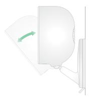
Note: To unmount your Essential Indoor Camera, slide the camera up until you hear an audible click, then pull the camera away from the wall plate.
