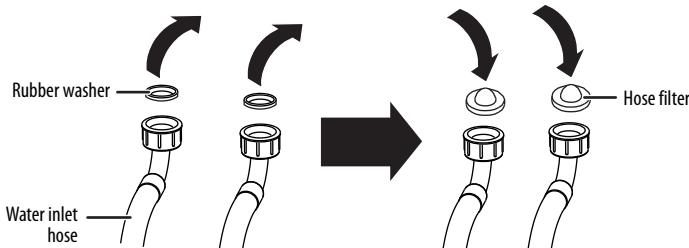
2 Tighten the hose and faucet fittings by hand until they are snug. Tighten them an additional two-thirds of a turn with pliers or a wrench. Pull the water inlet hoses downwards to make sure that they are connected securely.
