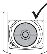
Washer is level - the water touches the leveling circle all the way around.
