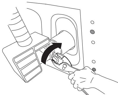
4 Connect the ends of the water supply hoses to the water supply intake connections at the top of your washer. Make sure that the rubber washers are in place. The water supply hose connected to the hot faucet must be connected to the hot water supply intake and the water hose connected to the cold faucet must be connected to the cold water supply intake.
