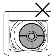
Washer not level - the water does not touch the leveling circle all the way around.
