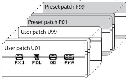
Built in to its memory, the GT-1 has 99 (starting from U01) user patches that can be overwritten, and 99 preset patches (starting from P01) that cannot be overwritten.
