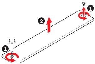
3. If you install 2280 SSD, use the included EZ M.2 Clip II Remover. Place the included EZ M.2 Clip II in the slot, use the remover to screw it in by turning it clockwise, and secure it. Skip this step if you install 22110 SSD.
