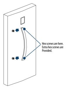
4 Place the door handle over the heads of the screws, then tighten the hex screws.
