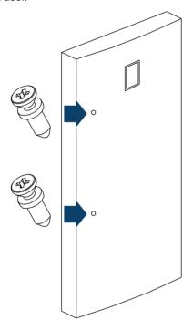
3 Loosen the hex screws on top and bottom of the handle with the hex wrench (provided) so that you can fit the handle over the extended head screws in the door.
