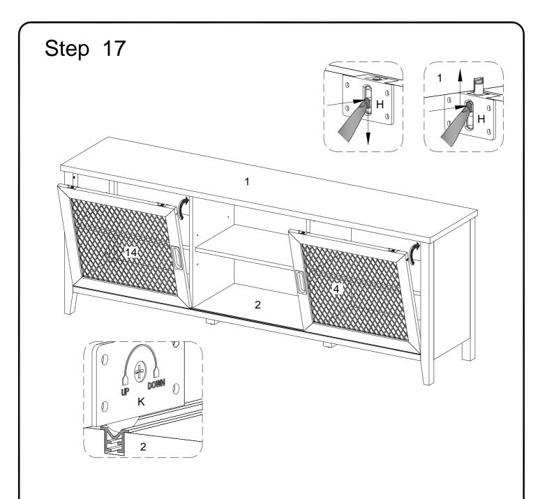
Pick up the doors (4,14), and fit the pulley (K) over the slider rails on the bottom panel (2) ,then place the doors (4,14) into top panel (1) , till it click into pulley (H) as per diagram.
