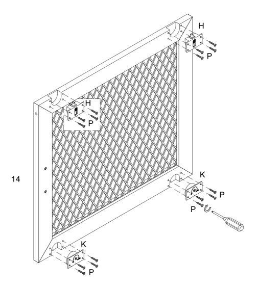
Using screw (P) secure pulley (K,H) into part (14) with Philips head screwdriver as per diagram.
