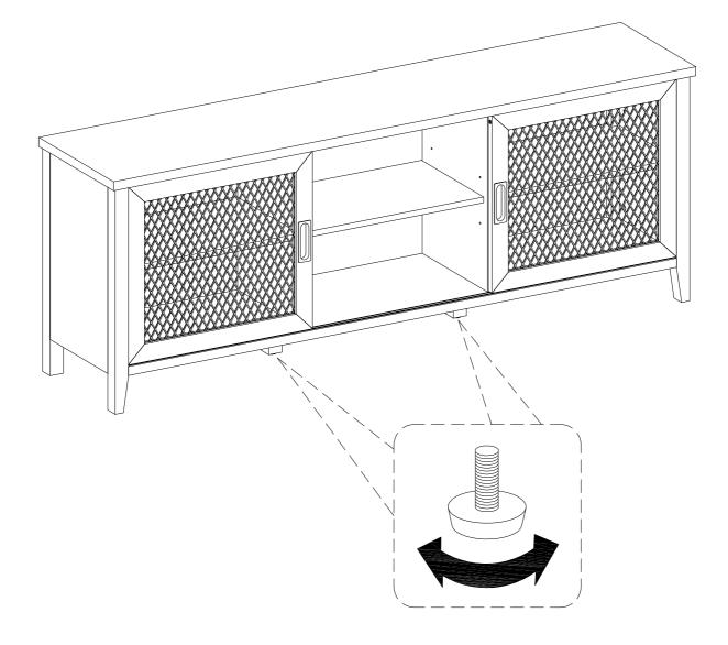
If necessary adjust the pre-attached floor levelers to level the unit .
