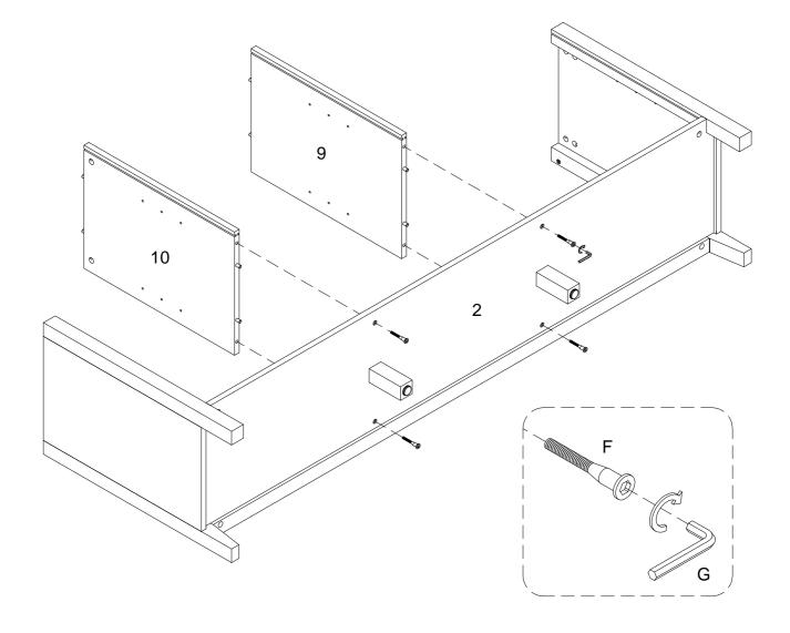
Using bolt (F) secure part (2) into parts (9,10) with hex key (G) as per diagram.
