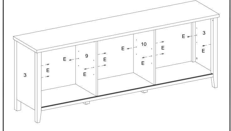
Insert shelf support pin into parts (3,9,10) as per diagram.
