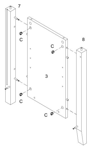
Using cam lock secure parts (5,6,7,8) into part (3) with Philips head screwdriver as per diagram.
