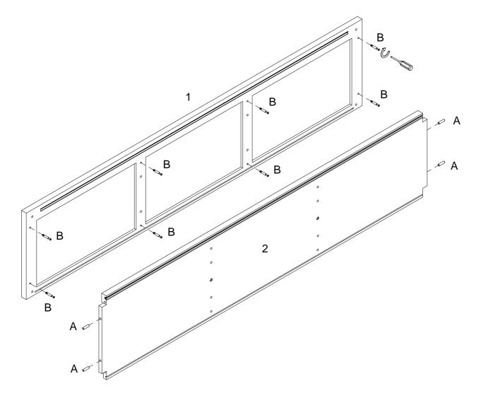
Insert wooden dowel (A) into part (2), using cam bolt (B) into part (1) with Philips head screwdriver as per diagram.
