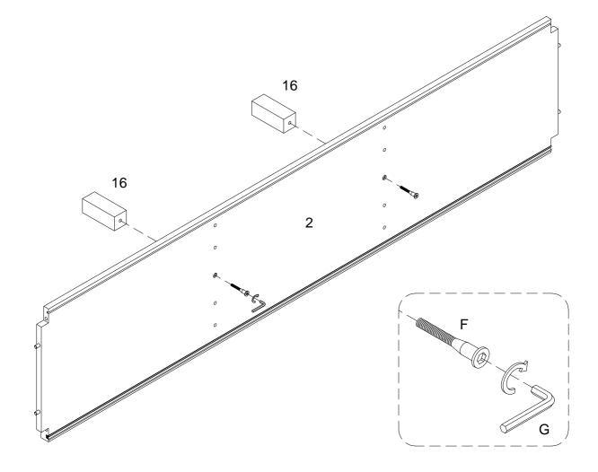
Using bolt (F) attach part (2) into part (16) with hex key (G) as per diagram.
