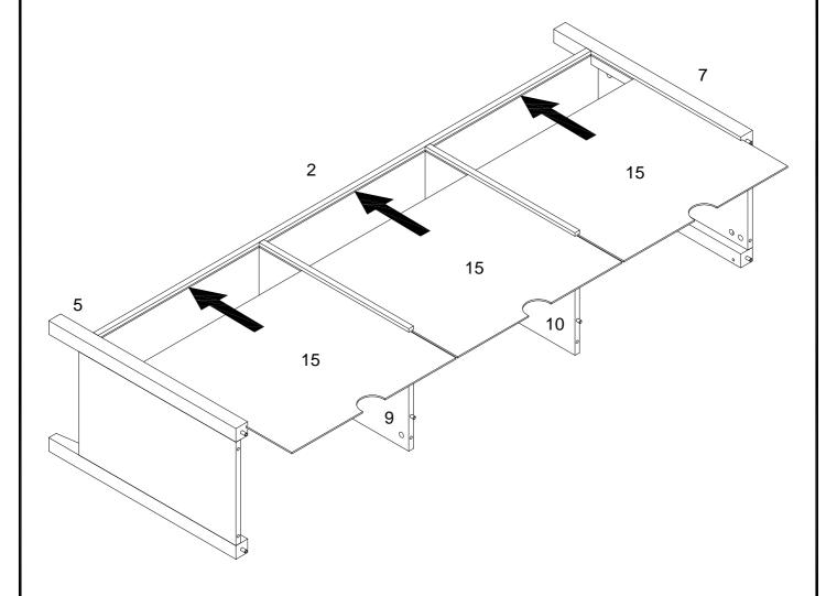
Put part (15) into parts (2,5,7) as per diagram.
