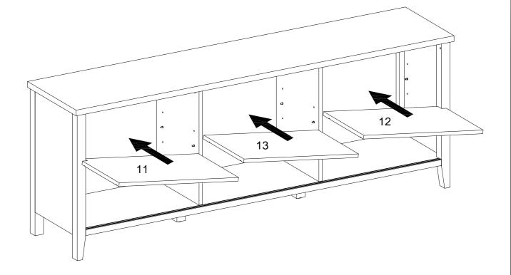
Put parts (11,12,13) into cabinet as per diagram.
