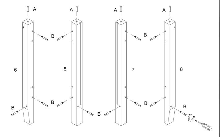
Insert wooden dowel (A) into parts (5,6,7,8), using cam bolt (B) secure parts (5,6,7,8) with Philips head screwdriver as per diagram.
