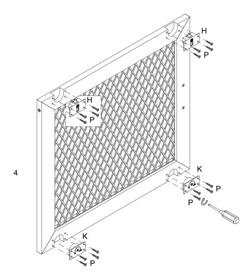
Using screw (P) secure pulley (K,H) into part (4) with Philips head screwdriver as per diagram.
