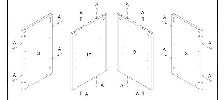
Insert wooden dowel (A) into parts (3,9,10) as per diagram.
