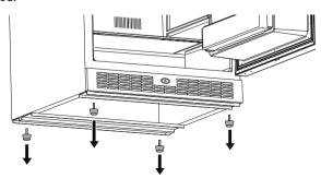
3 Install the non-locking casters on the back of the appliance.
