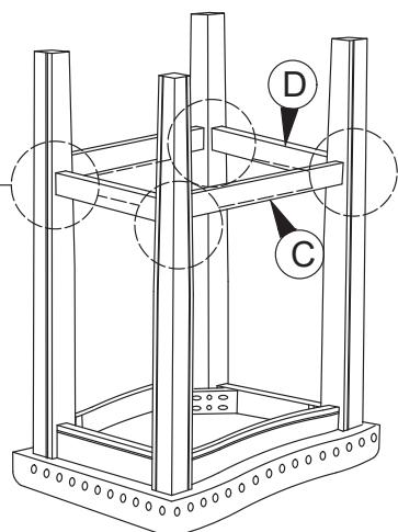
**EN:** Tighten part(C) and part(D) completely!
