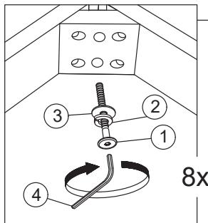
**EN:** Tighten part (A) with part (B) completely after alignment is done.
