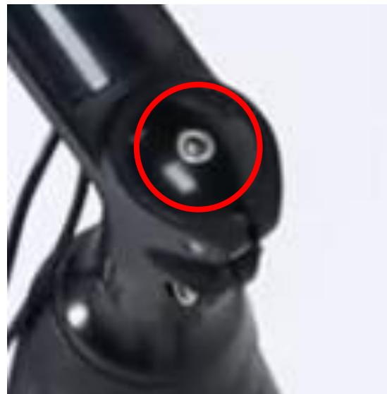
Step 3: After the handlebar is properly aligned and the top screw is tightened, tighten the 2 side screws, as indicated in the pictures.
