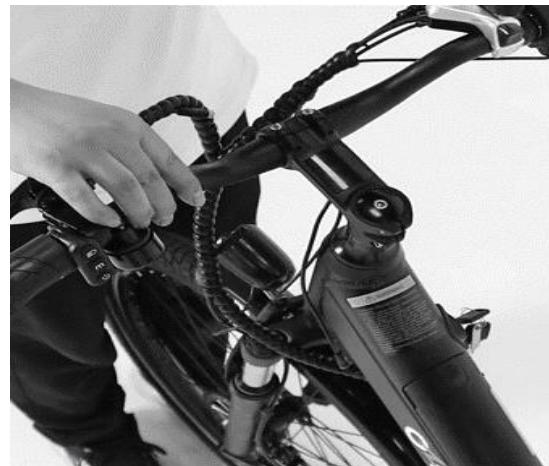
Step 2: Tighten the top screw.
