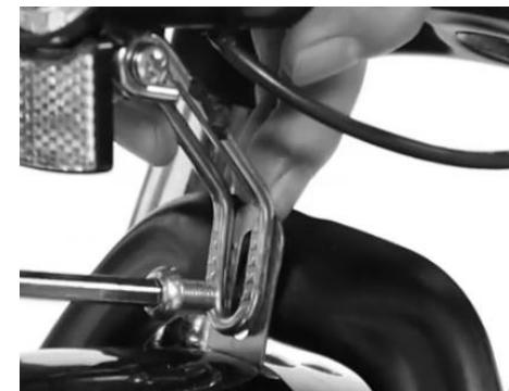
Step 4: Align the fender “U” brace arms to the tabs on the rear side of the front fork
