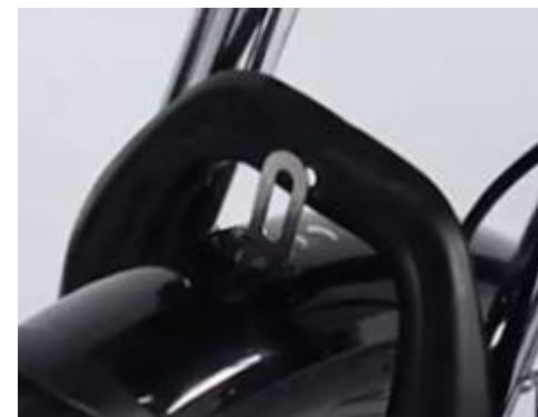
Step 3: Move headlight into place and use the screw to attach the headlight and fender.
