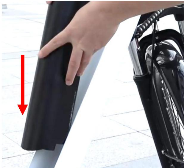
Step 3: Reinstall battery by sliding the bottom of the battery into the battery compartment and sliding the battery in a downward motion locking it into the battery compartment.
