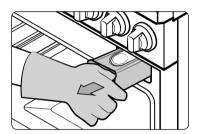
Locate the water reservoir. The water reservoir is on the right side of the oven, just above the oven opening. Push Open/Close reservoir on the control panel. The oven ejects the water reservoir. Grasp the front of the reservoir, and then slide it out to remove it.
