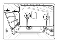
Put the top of the Ladder Rack back into the two support holes in the oven wall.
