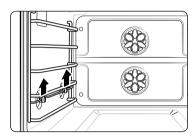
Grasp the Position 2 rack guide, and then lift the Ladder Rack straight up. This frees the Ladder Rack from the two supports on the oven wall.
