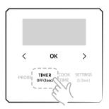
3. Press the **Timer** and **Oven light** button simultaneously for 3 seconds to display "**OK**". Once "**OK**" appears, the oven control no longer beeps or displays any further changes.
