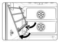
2. Rotate the Ladder Rack towards the oven wall.
