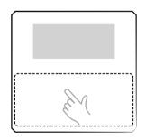
To activate the control panel, touch the lower area of the screen to wake it up. User preferences are available in this mode including the timer and/or Child Lock.
