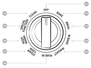
The Modes are printed on the knob itself. To select a mode, turn the knob so that the mode you want is aligned with the line on the knob frame.
