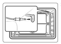
Insert the temperature probe plug into the socket on the right side wall of the oven.
