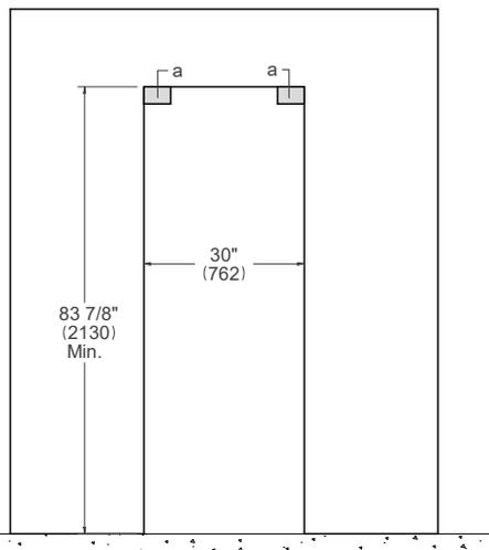
(a) Area to be left clear for the anti-tipping brackets – 3 1/2x5" (82x127mm)
