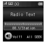
RBDS (Radio Broadcast Data System) mode provides additional functionality to FM radio reception by transmitting encoded analog information with the FM radio signal. This signal is decoded by an RBDS receiver and can provide a range of informational features including the station's name. The RBDS text is usually centered. When the text fills the display, it begins scrolling. When receiving an RBDS signal, the "RBDS" icon appears on the display.
