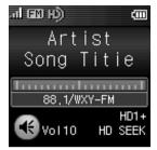
The HD Radio mode is the new, digital mode. Many HD Radio stations have several sub-channels called "Multicast Channels." When receiving an HD Radio signal, the "HD" icon and the channel number appear on the display.
