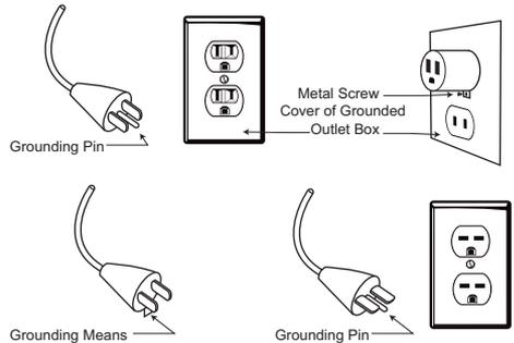
**WARNING:** It is normal for the power cord to feel warm to the touch. However, a loose fit between the outlet and the plug may cause overheating of the plug. If this occurs, try inserting the plug into a different outlet. Contact a qualified electrician to inspect the original outlet for damage.
