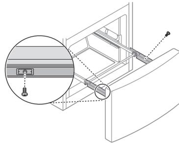
5 Grip both sides of the drawer and pull it up to remove it from the rails.
