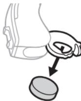
**TIP:** You can use the magnetic end of the hearing aid brush to easily remove the battery.
