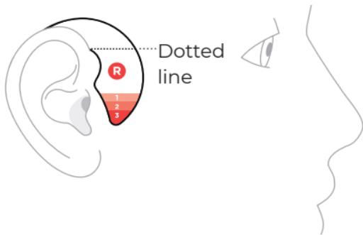
Make sure that the dotted line near the top of the tool is level and aligned with the top of your ear.
