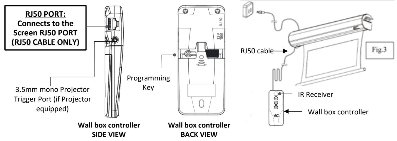
**4. Wired 5-12 volt trigger:** Requires a 3.5mm to 3.5mm mono cable (not included)
