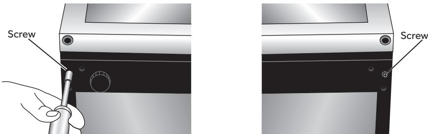
6. Using the three hex-head screws removed earlier, reinstall the bottom hinge on the opposite side.
