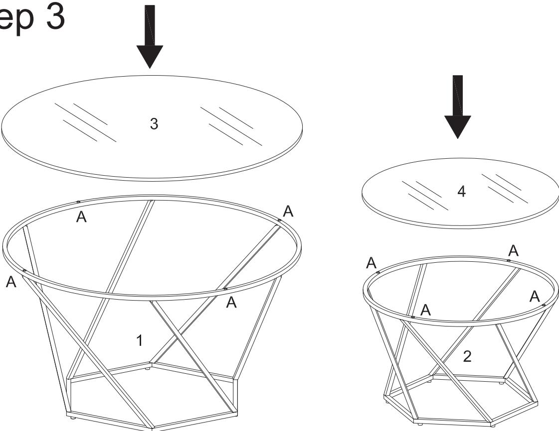
Place the glass table top (3,4) on top of the metal base (1,2) carefully as per diagram.
