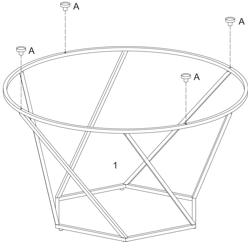
Insert the rubber suction cups (A) to the metal base (1).
