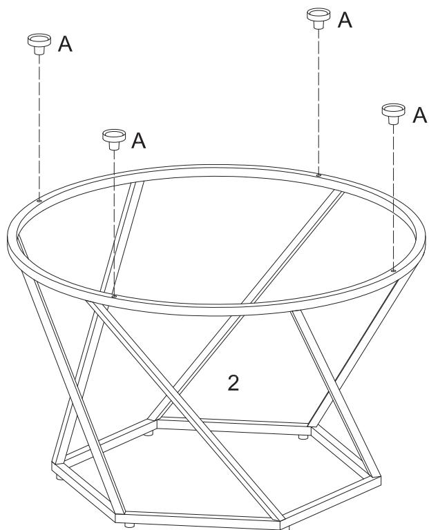
Insert the rubber suction cups (A) to the metal base (2).
