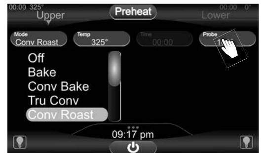
If the timer is set and probe is inserted, the timer is disabled. Probe temp flashes every 10 seconds between actual temp and set temp.
