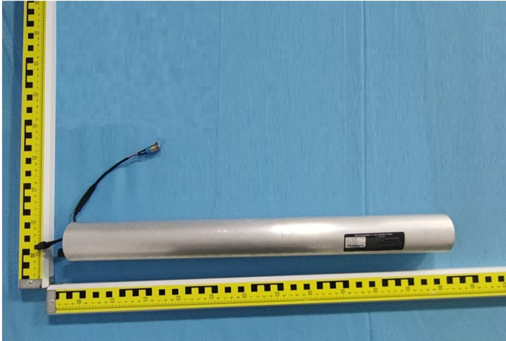
Picture 18. Front view of battery (Remark: internal battery assembly were encapsulated in this metal tube)
