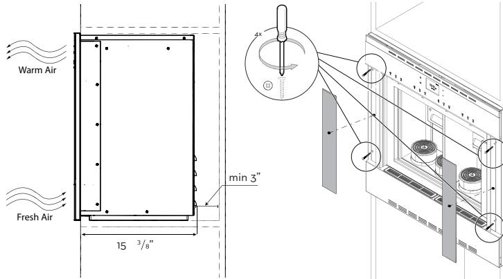
A. Insert 4 #3.5mm x 30mm screws in the predrilled holes
