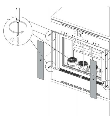
A. Insert 4 #3.5mm x 30mm screws in the predrilled holes
