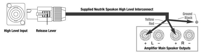
• For differential (i.e. fully balanced) amplifiers using one REL, simply use the standard connecting scheme with the exception of NOT connecting the black wire to a negative speaker terminal. Instead, it should first be connected to a ground lug or chassis screw. Should hum occur using this method, the black wire should be allowed to "float" or hang down without connection to ANY terminal.
