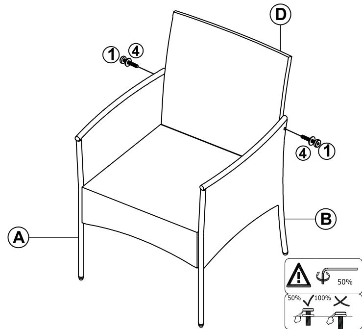
**EN** Connect the parts of the Back Frame (D) to Right Arm Frame (A) and Left Arm Frame (B) completed in STEP 3 with Bolts (1) & Washers (4)
