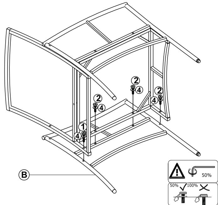
**EN** Connect part from STEP 2 to Left Arm Frame (B) with Bolts (1), (2) & Washers (4)
