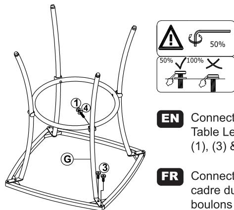
**EN** Connect part from STEP 7 & Table Leg Frame (G) with Bolts (1), (3) & Washers (4)
