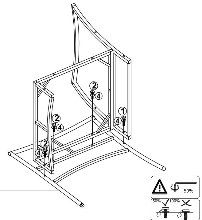
**EN** Connect Back Frame (D) to Seat Frame (C) with Bolt (2) & Washer (4)
