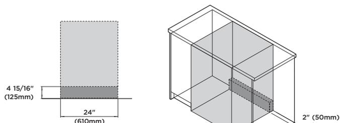
SERVICE OUTLET AT REAR EXTENDS BOTH SIDES, HOSES AND CORDS CAN BE ROUTED TO EITHER OR BOTH.
