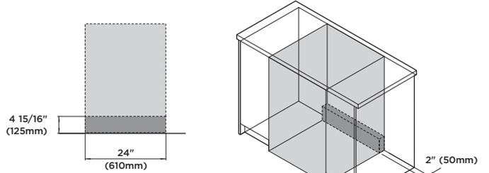
SERVICE OUTLET AT REAR EXTENDS BOTH SIDES, HOSES AND CORDS CAN BE ROUTED TO EITHER OR BOTH.
