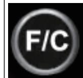
The Temperature Switch Button is used to change the temperature readout on the LED Screen. Press the button to switch to Celsius (°C) to Fahrenheit (°F), as preferred. Default is set to Fahrenheit.
