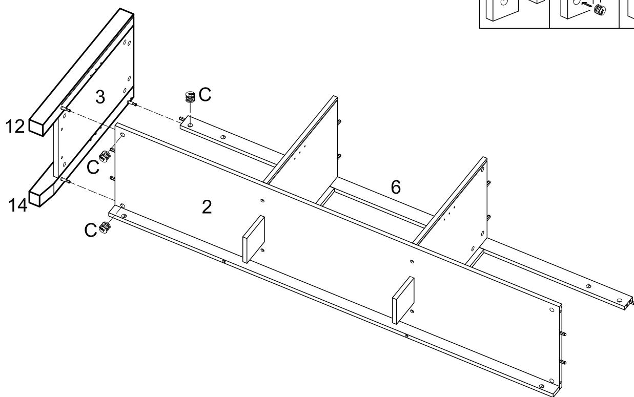
Attach panel (3) with legs (12,14) to the assembly from the previous step using cam bolts and dowels as guides. Insert cam locks (C) into panel (2) and slat (6) and tighten with a screwdriver.
