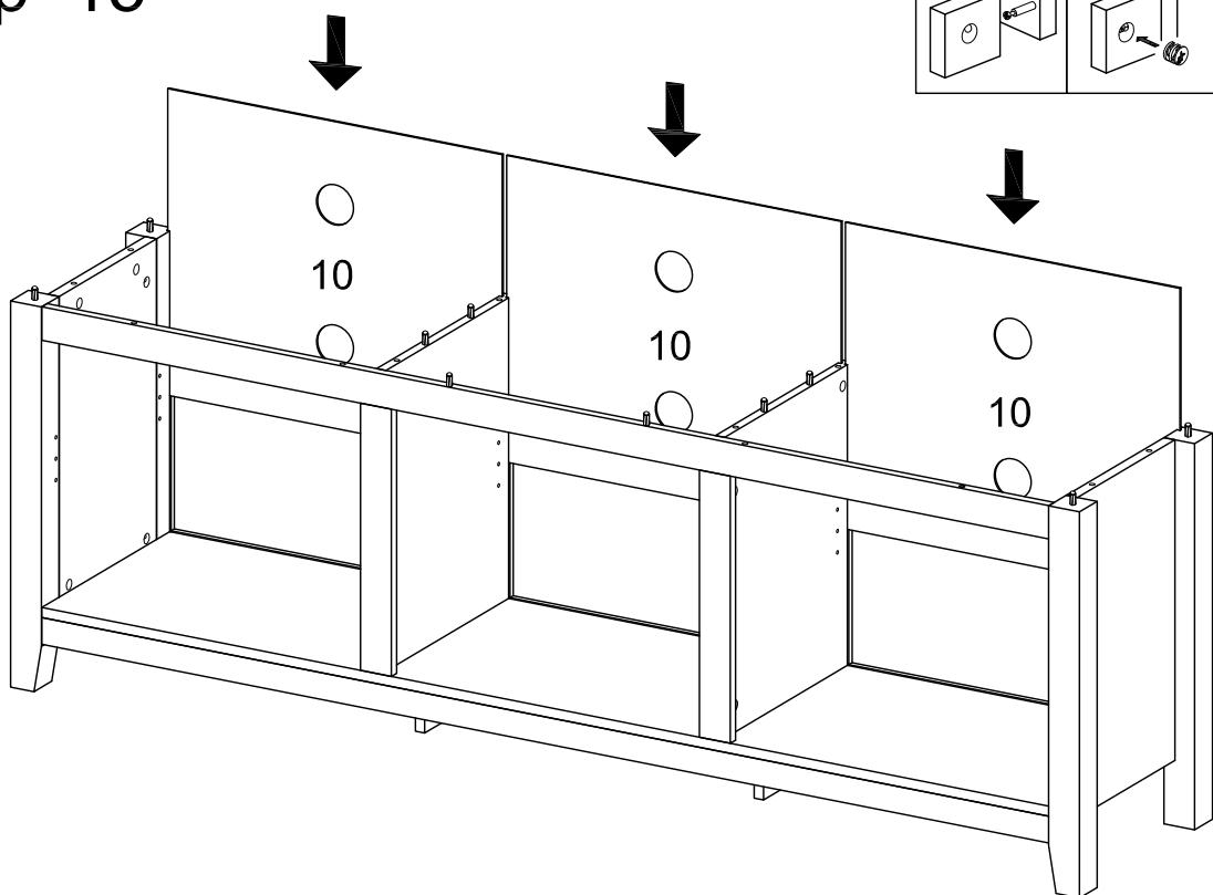
Carefully slide panels (10) into place along the back of the assembly.
