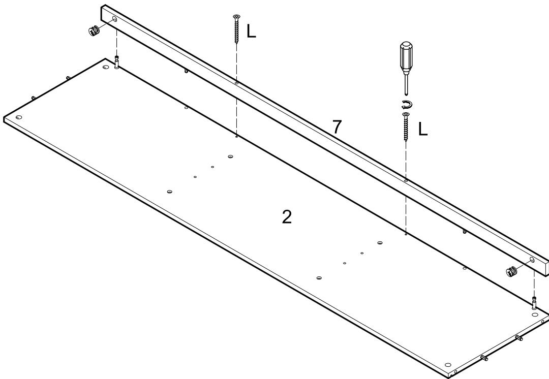
Attach slat (7) to panel (2) using cam bolt as guides. Insert cam lock (C) into slat (7) and tighten with a screwdriver. Secure screw (L) to slat (7) to panel (2).
