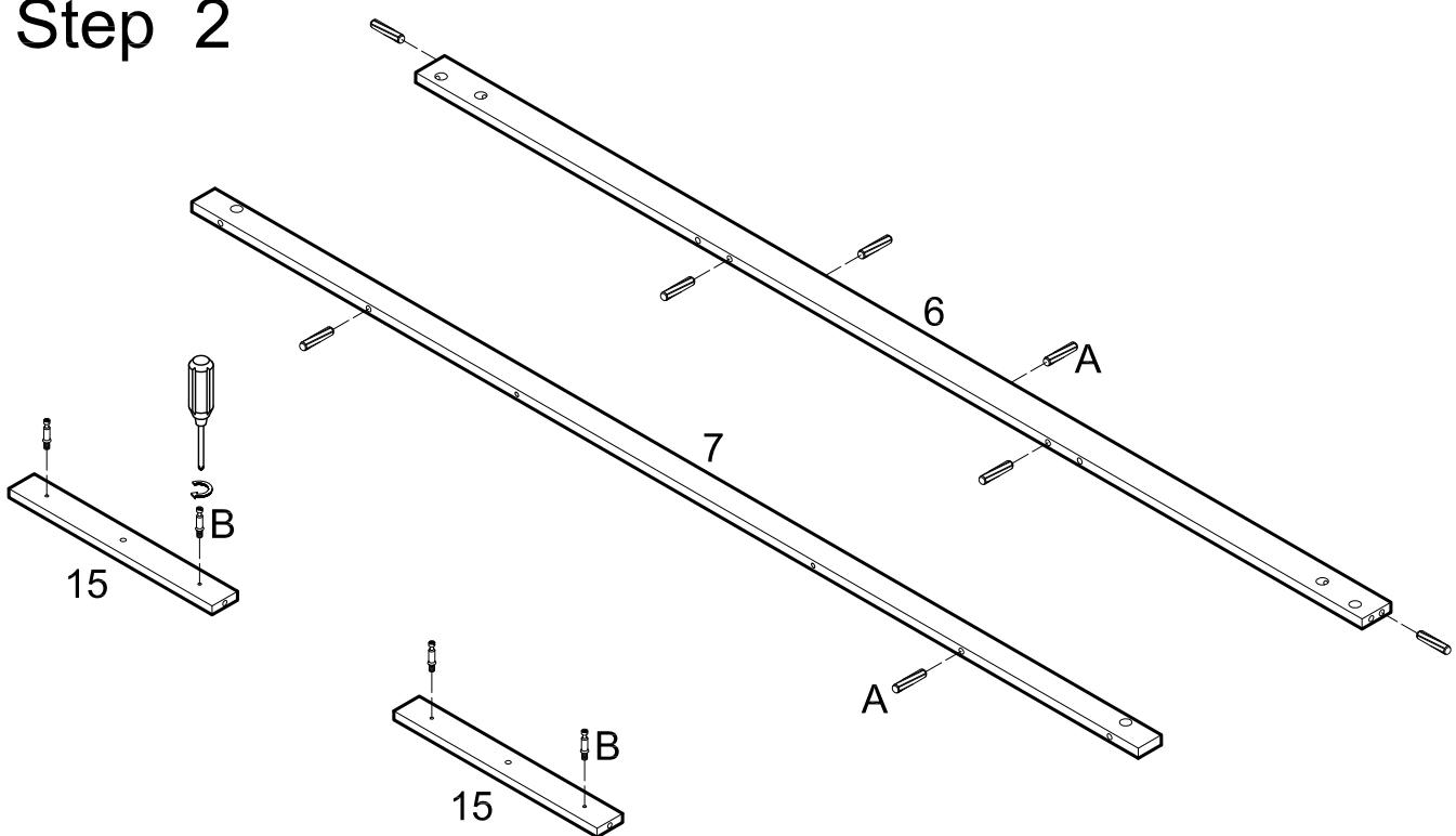
Insert dowels (A) into slats (6,7). Screw cam bolts (B) into slats (15).
