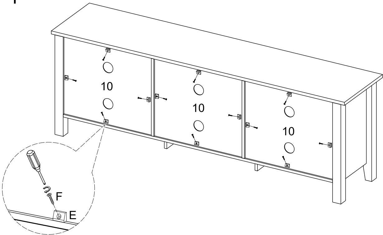
Secure panels (10) with plastic wedges (E) and screws (F).
