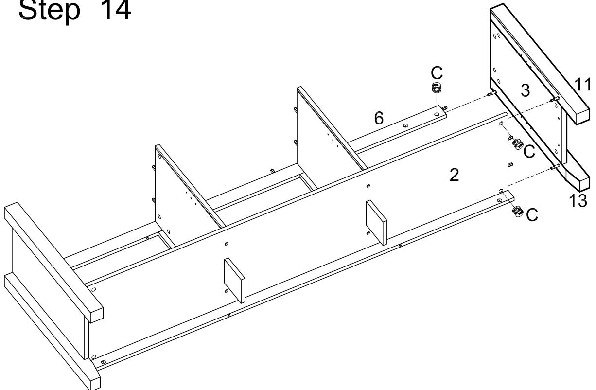
Attach second panel (3) with legs (11,13) to the assembly from the previous step using cam bolts and dowels as guides. Insert cam locks (C) into panel (2) and slat (6) and tighten with a screwdriver.
