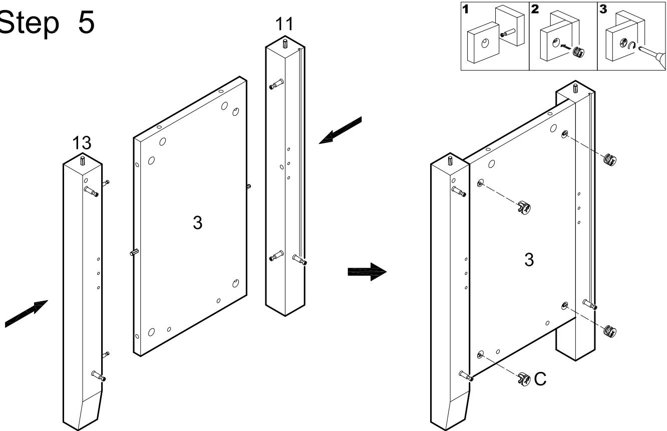
Attach legs (11,13) to panel (3) using cam bolts and dowels as guides. Insert cam locks (C) into panel (3) and tighten with a screwdriver.
