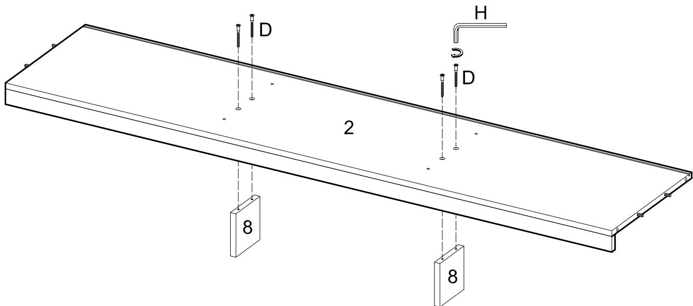
Attach support legs (8) to panel (2) using bolts (D). Tighten bolts (D) with wrench (H).
