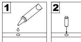
In future assembly steps when dowels are necessary to attach assembly parts together , place a small amount of glue on the end of the dowel before attaching parts together . Wipe away excess glue immediately.
