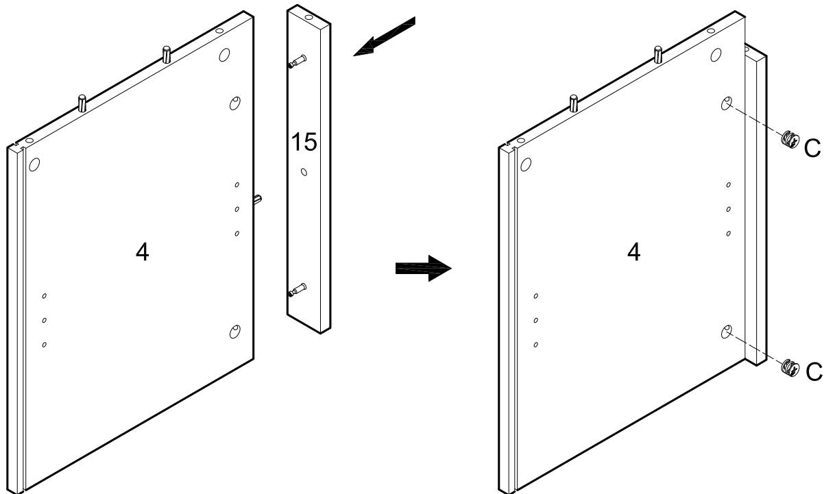
Attach slat (15) to panel (4) using cam bolts and dowel as guides. Insert cam locks (C) into panel (4) and tighten with a screwdriver.
