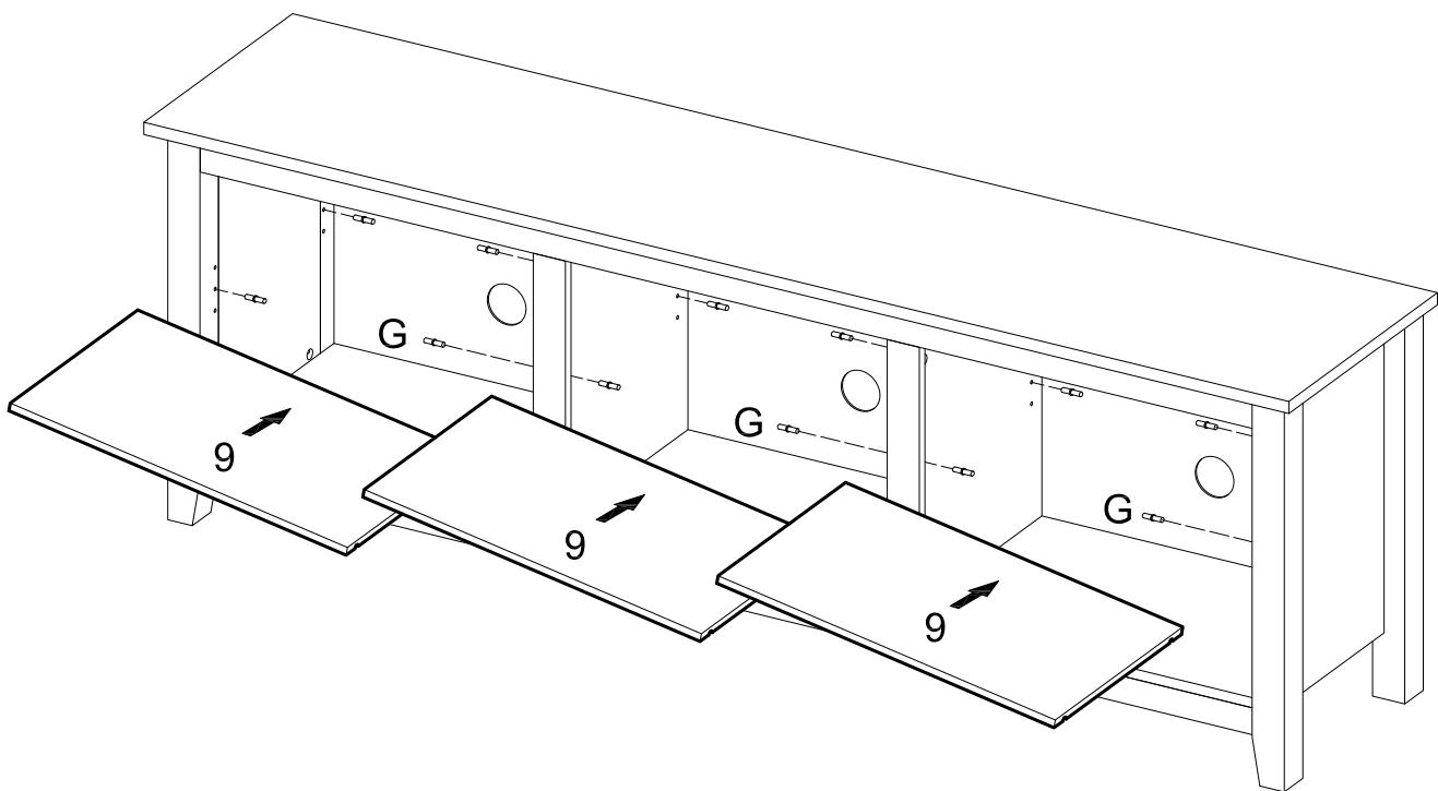
Insert shelf support pins (G) into the assembly at desired shelf heights. Carefully place shelves (9) on shelf support pins (G).
