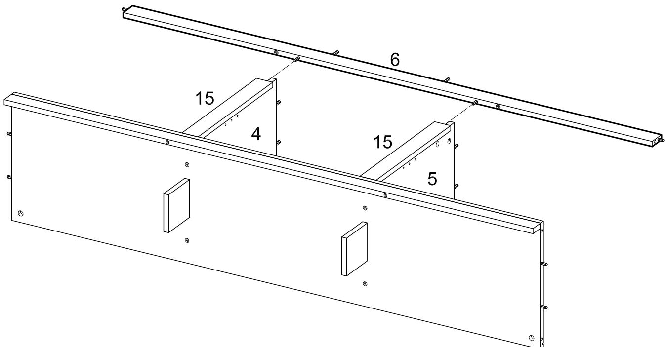
Attach slat (6) to slats (15) using dowel as guide.
