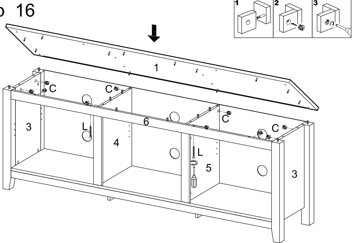
Carefully attach panel (1) to the assembly using cam bolts and dowels as guides. Insert cam locks (C) into the assembly as shown above and tighten with a screwdriver. Secure screw (L) to slat (6) to panel (1).
