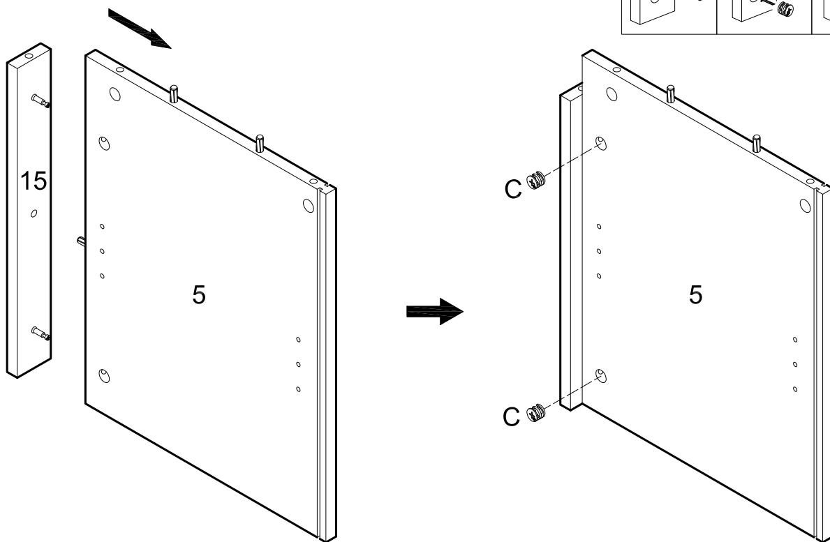
Attach slat (15) to panel (5) using cam bolts and dowel as guides. Insert cam locks (C) into panel (5) and tighten with a screwdriver.
