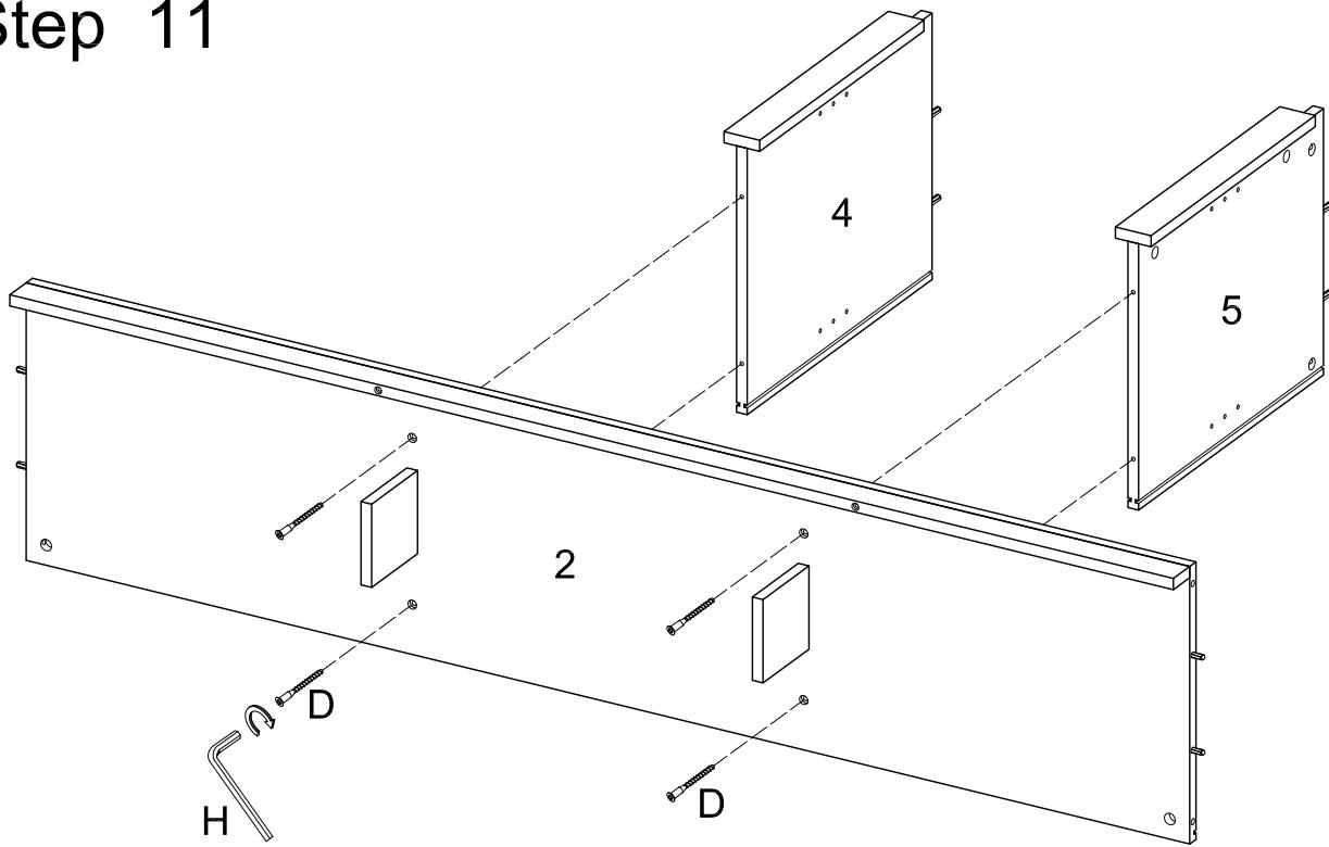
Attach panel (4,5) to panel (2) using bolts (D). Tighten bolts (D) with wrench (H).
