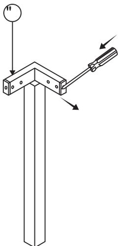
Insert a screwdriver into the plastic plug hole and pry out.
