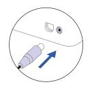
First, connect the AC adapter jack to the printer adapter port.
