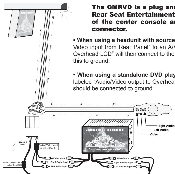
**Note:** This cable is intended for use in conjunction with an OS-4 to retain all safety and convenience systems. The vehicle should be equipped with a Panasonic Overhead LCD and IR system, in which the DVD player was part of the AM/FM/CD receiver. The OS-4 is needed to power the IR headphone system.
