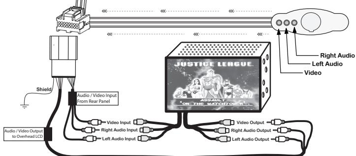
**Note:** This cable is intended for use in conjunction with an OS-4 to retain all safety and convenience systems. The vehicle should be equipped with a Panasonic Overhead LCD and IR system, in which the DVD player was part of the AM/FM/CD receiver. The OS-4 is needed to power the IR headphone system.
