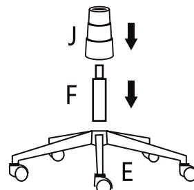
Insert the gas cylinder into the base, followed by the plastic cover.
