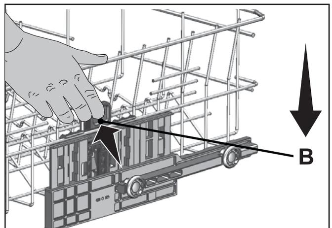
**i** The movement mechanism may not function properly if the upper basket is overloaded or if the weight distribution is not balanced. In heavier conditions, there is the risk of falling one level down.
