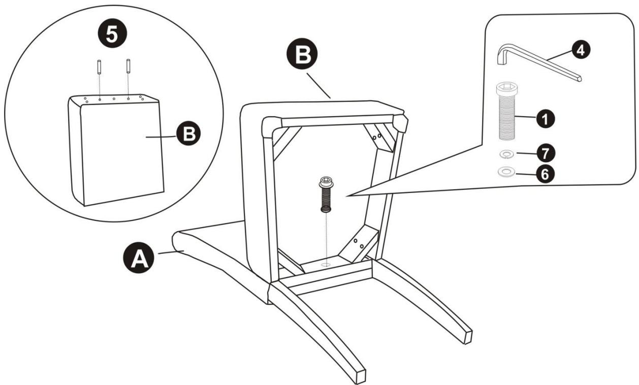
Insert Dowels (5) into pre-drilled holes on Seat (B).
