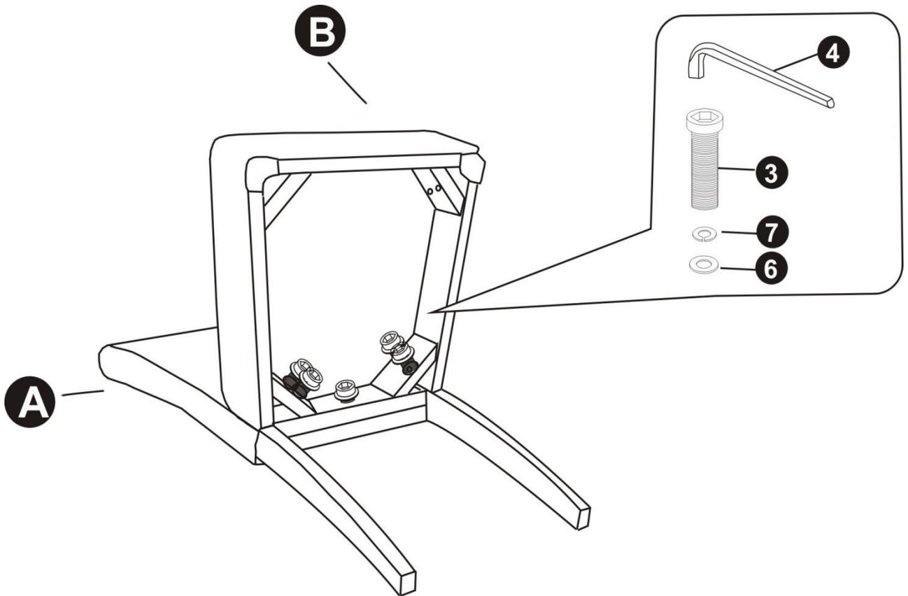
Secure Seat (B) to Chair Back (A) using Allen Keys Screws (3) and four Washers each of (6) and (7).
