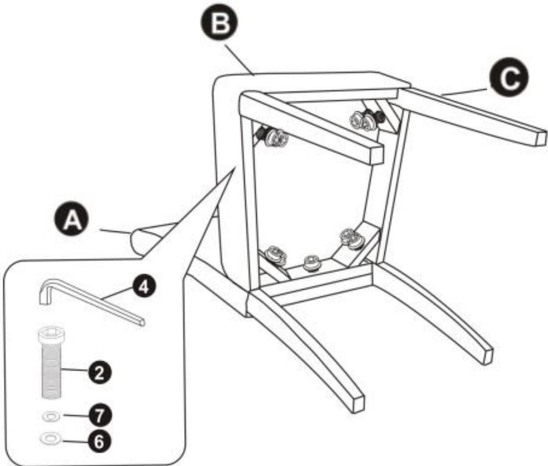
Attach Front Leg (C) to Seat (B) using Allen Keys Screws (2) and four Washers each of (6) and (7).
