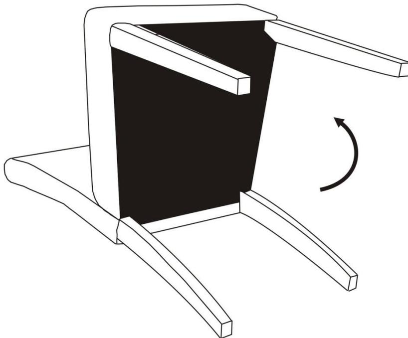
Attach fabric with velcro to bottom of Seat.
