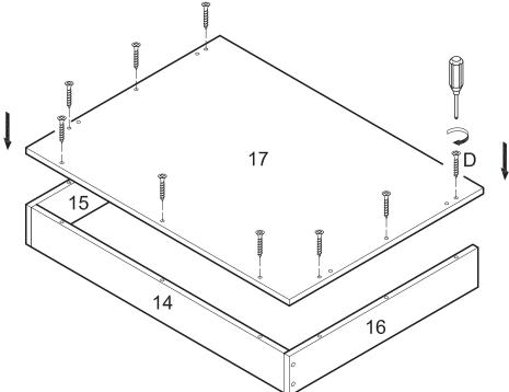
Attach drawer bottom (17) to drawer sides (15,16) and drawer back (14) using screws (D). Tighten screws (D) with a screwdriver.
