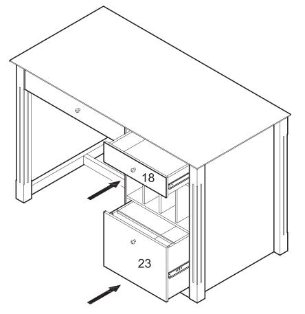
Carefully slide the remaining drawers into place. Note that you will need to align the metal tracks of the drawers with those on the desk to slide the drawers into place.
