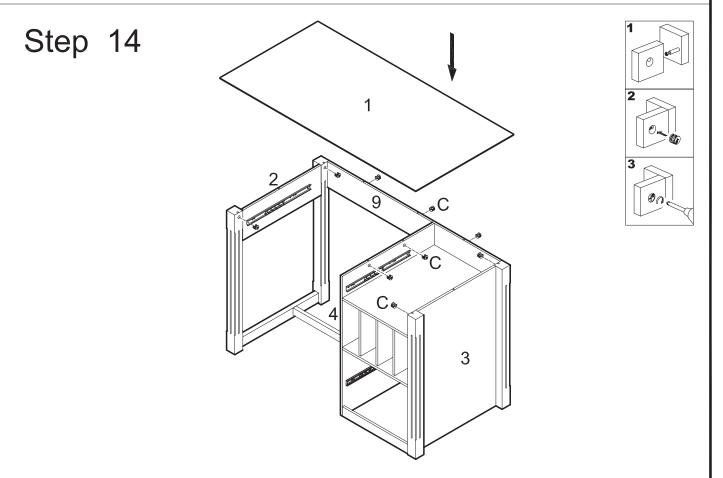
Insert cam locks (C) into panels (2,3,4) and slat (9). Fit desk top (1) into place using cam bolts and dowels as guides. Tighten cam locks (C) with a screwdriver to secure desk top (1).
