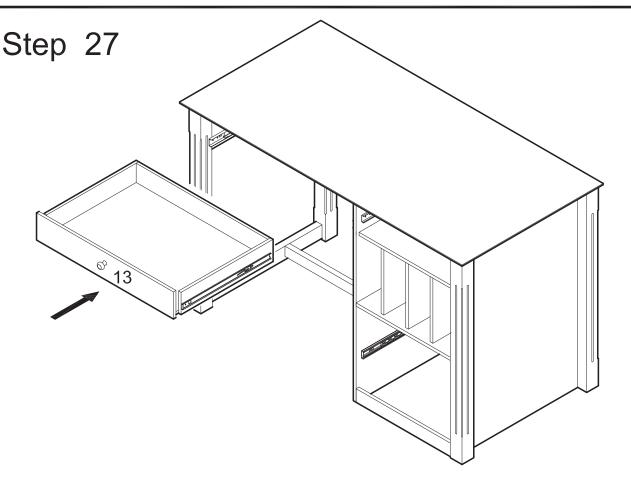
Carefully slide the drawer into the desk assembly. Note that you will need to align the metal tracks of the drawer with those on the desk to slide the drawer into place.
