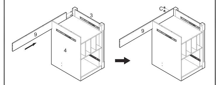
Fit slat (9) onto panel (3) using cam bolts as guides. Insert cam locks (C) into slat (9) and tighten with a screwdriver.
