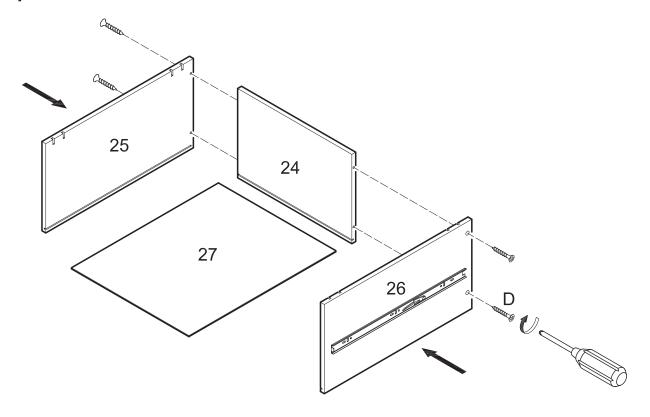
Attach drawer sides (25,26) to drawer back (24) using screws (D). Carefully slide drawer bottom (27) into place along the grooves of the drawer assembly.
