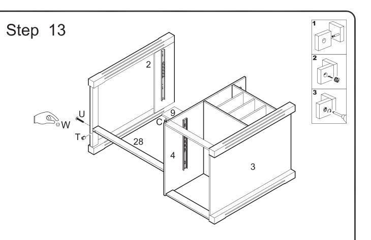
Insert cam locks (C) into slat (9) and tighten with a screwdriver. Note that two cam locks (C) will be inserted into slat (9). Insert barrel nut (T) into slat (28). Secure slat (28) to panel (2) using bolt (U). Note that bolt (U) will screw directly into barrel nut (T). Cover bolt (U) with cap (W).
