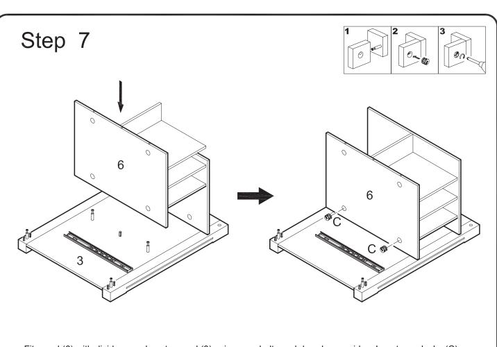
Fit panel (6) with divider panels onto panel (3) using cam bolts and dowels as guides. Insert cam locks (C) into panel (6) and tighten with a screwdriver.
