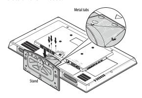
3 Secure the stand with the provided M4 × L14 mm screws (26" – 1 screw 32" – 3 screws).
