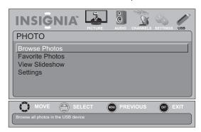
3 Press ▲ or ▼ to highlight Favorite Photos, then press OK/ENTER. A thumbnail index of your favorite photos opens with a control bar at the bottom of the screen.
