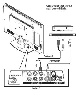
3 Connect an audio cable to the L/R (audio in) jacks on the back of your TV and to the L/R AUDIO OUT jacks on the S-Video device.
