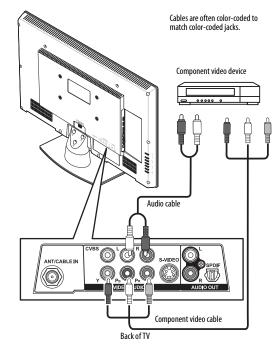
3 Connect an audio cable to the L/R (audio in) jacks on the back of your TV and to the L/R AUDIO OUT jacks on the component video device.
