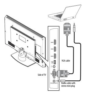
3 Connect an audio cable with stereo mini plug to the VGA AUDIO IN jack on the side of your TV and to the LINE OUT or AUDIO OUT jack on the computer.
