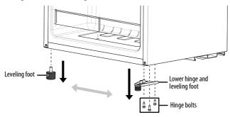
**9** Attach the lower hinge and leveling feet to the opposite sides of your cooler.
