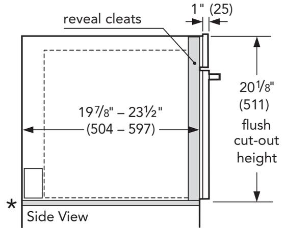
**NOTE:** \* Flush installation requires a 5/16" (8 mm) high x 28<sup>1</sup>/<sub>2</sub>" (724 mm) wide x 22<sup>1</sup>/<sub>2</sub>" (571 mm) deep baseplate underneath the unit body.
