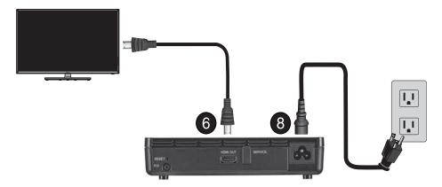
**Note**: It's best to connect the AC power cord directly to a wall outlet. Using a surge protector with noise filtering may decrease the data rate and may affect the quality of the signal.
