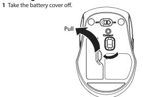
2 Insert the included AAA batteries into the battery compartment. Make sure that the + and - signs match the symbols on the ribbon in the compartment.
