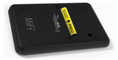
**2** Pull the plastic tab out in the direction of the arrow.
