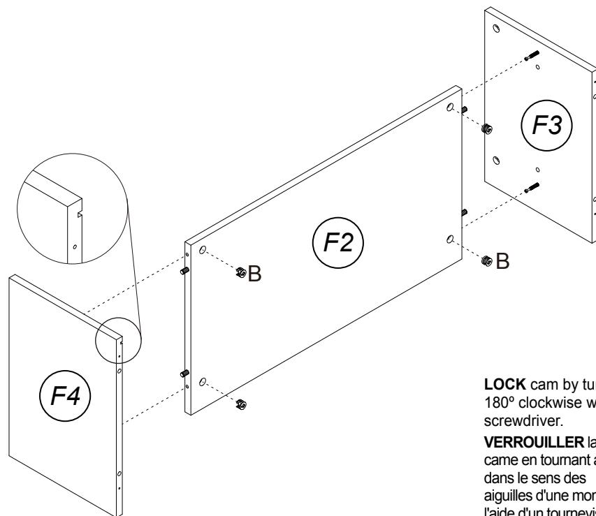
**LOCK** cam by turning 180° clockwise with a screwdriver.
