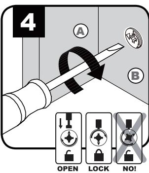
**LOCK** cam by turning 180° clockwise with a screwdriver.
