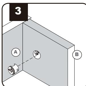
Insert Cam into side panel **B** Making sure ▲ points towards face panel **A**.
